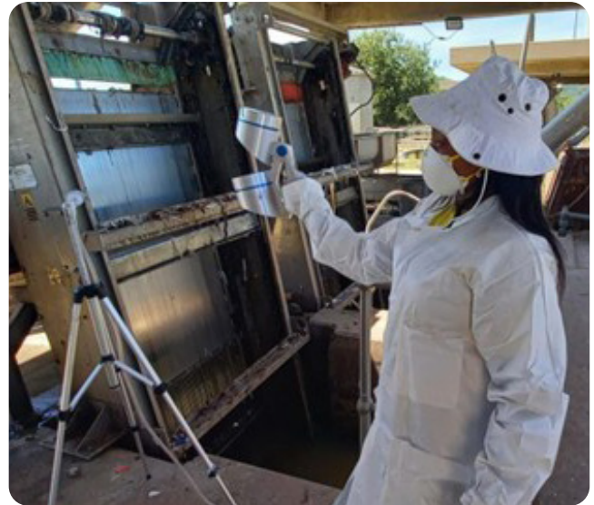
A postgraduate student conducting air sampling near inlet screens at a wastewater plant.
