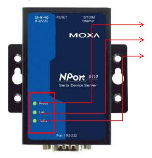
Power indicator (Green Light) TCP/IP indicator (Green Flashing light) Rx/ indicator (Orange flashing light)
